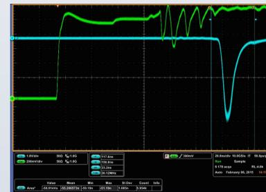
The cross-talk is further reduced with introduction of a grounding plane and baffling between LEDs. Pictured right is the clock (green) and pulse (blue).
