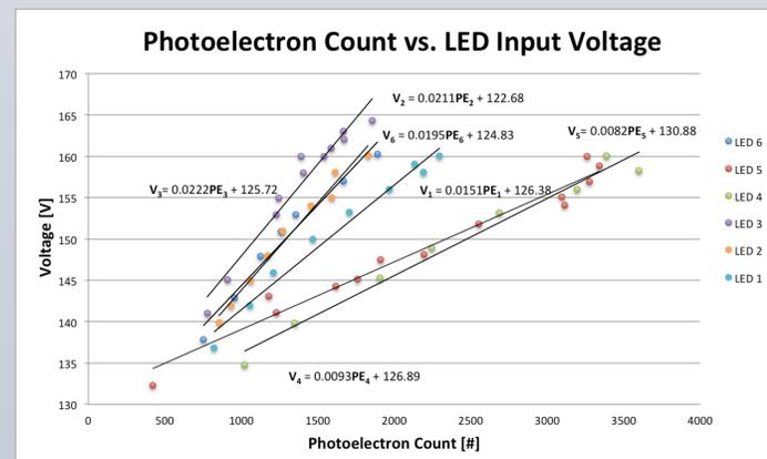
To first order, we assume linearity in the PMT. There seems to be a convergence at ~800 PE for 135V. This isn't enough PEs to work with, so we examine optical fiber ends, improve cutting techniques, increasing PE counts by ~200%.
