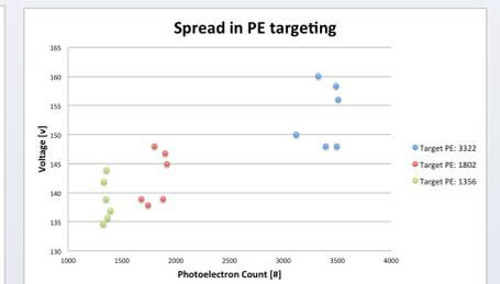
The cause of spread in voltage, even with PE targeting, is thought to be due to artificial widening/narrowing of peaks, or fluctuation of the peak itself.
