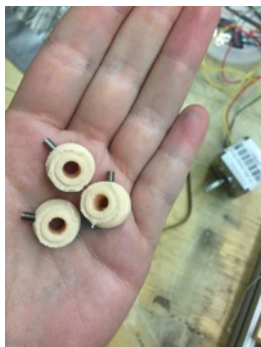
Figure 5: Tapped pulleys, added set screws, so no sliding.
